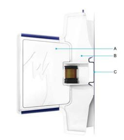
Module (A) and base (B) form a unique combination. As a result of this, a module cannot be incorrectly positioned in a base.
