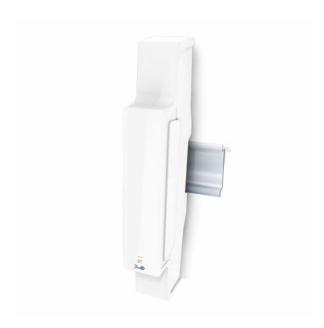
An Priva Blue ID S-Line ST Termination module can easily be slid onto the base of the last I/O module or controller. The system does not work without this module.
