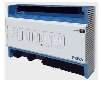
The Priva Blue ID C-Line MX34m Mix input/output module with manual override provides analogue outputs, software configurable inputs for analogue and digital use and controls output functions with a relay.
