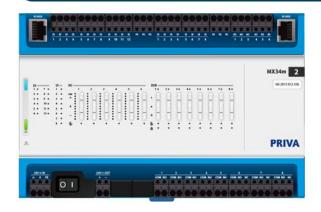
Priva Blue ID C-Line is build around a freely-programmable controller for process control and monitoring. The controllers and IO modules are diverse and flexible and can be used in countless environments, for instance in buildings.
