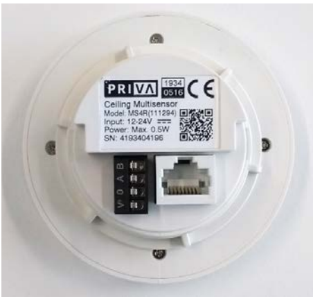
Rear side of the multisensor with connections
